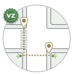
There are two types of formal Controlled crossing: Zebra, requiring vehicles to give way, and signals, requiring vehicles to stop. These should be used whenever safety of people crossing the street requires formal control.
