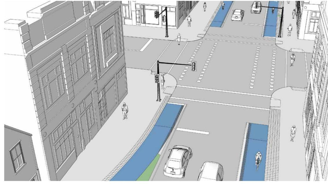
Unprotected intersections are intersections where cyclists are more exposed to traffic due to a lack of corner safety islands. Cyclists mix with vehicle traffic on the intersection and with pedestrian traffic where they cross the crosswalk.
