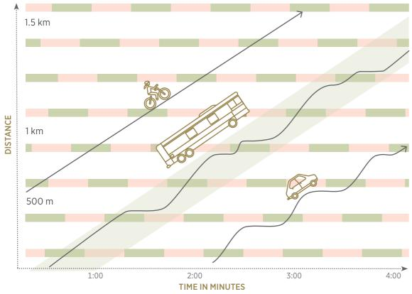
Low speed signal progressions create amenable environments for both bicycle green waves and bus or LRT priority streets.
