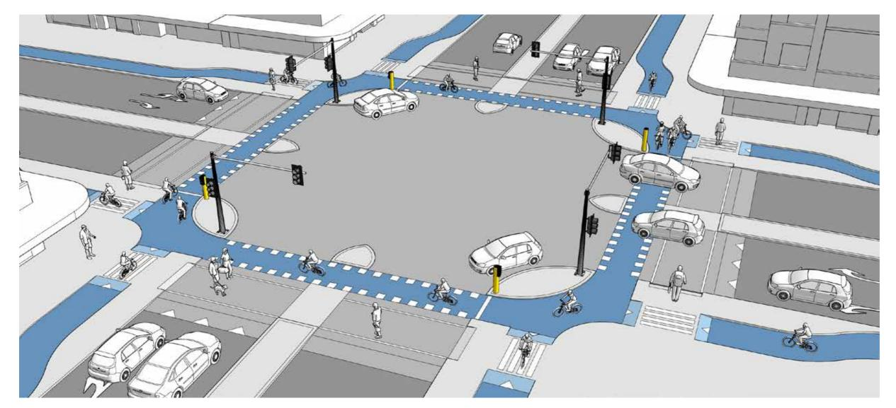
Protected intersections maintain the physical separation through the intersection, thereby eliminating the merging and weaving movements inherent in conventional cycle lane and shared lane design.
