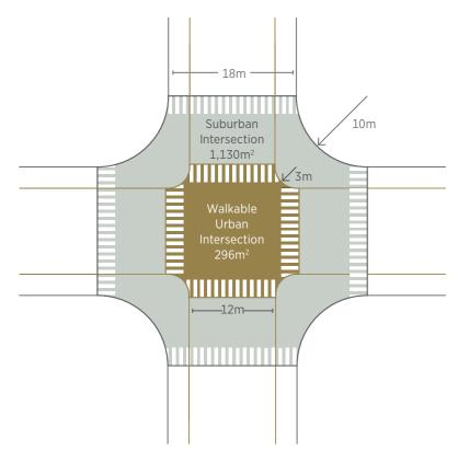
adequately respond to each other's movements and actions. Minimised kerb radii also benefit cyclists, as speeds of turning vehicles are reduced, thus reducing the risk of a turning motorist turning left across the path of a cyclist going straight across the intersection.
