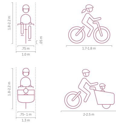
Minimum envelope for bike users is 1.0 m wide, allowing for some weaving for stability, especially uphill.
